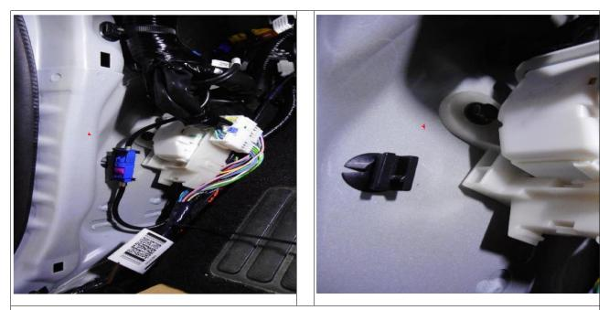
18. Disconnect the vehicle installation plug.
