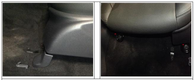
2. Slide the seat to the back. Remove the left plastic seat slider cover by pulling its upper part to the sides. Remove bolts fastening the seat sliders, using a 14mm socket wrench.
