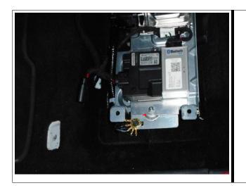
26. Press the connector over the CAN reader and the Pickup Design V8 Exhaust Sound System module ground wires, using pliers. Affix ground cables in the original spot, using a 10mm socket wrench.
