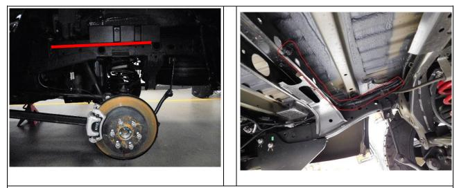
31. Run the loudspeaker wire along the inner side of the frame. Attach it to the original installation with cable ties.
