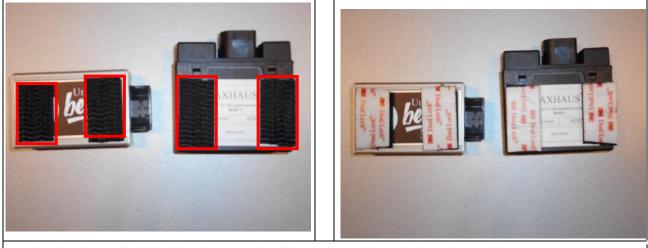
Attach stripes of 3M Dual Lock tape to the Bluetooth module and the main module.
