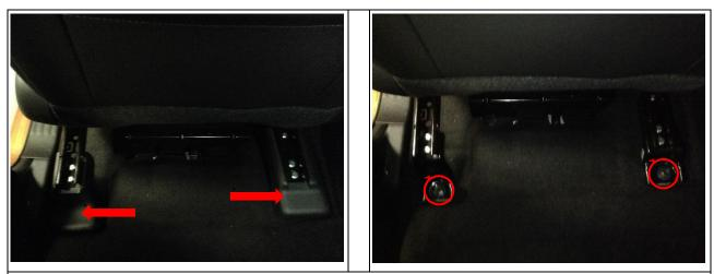
1. Slide the seat to the front. Remove plastic seat slider covers by pulling their bottom parts to the sides. Remove bolts fastening the seat sliders, using a 14mm socket wrench.
