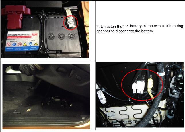
4. Lift the front part of the seat. Disconnect the plugs located under the seat base.
