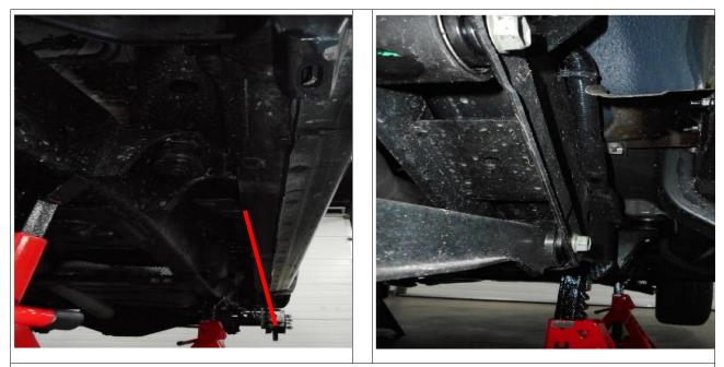
29. Run the loudspeaker wire along the vehicle frame, mounting it to the original installation with cable ties.30. Put the loudspeaker wire to the inner side of the frame. Attach it to the original installation with cable ties.
