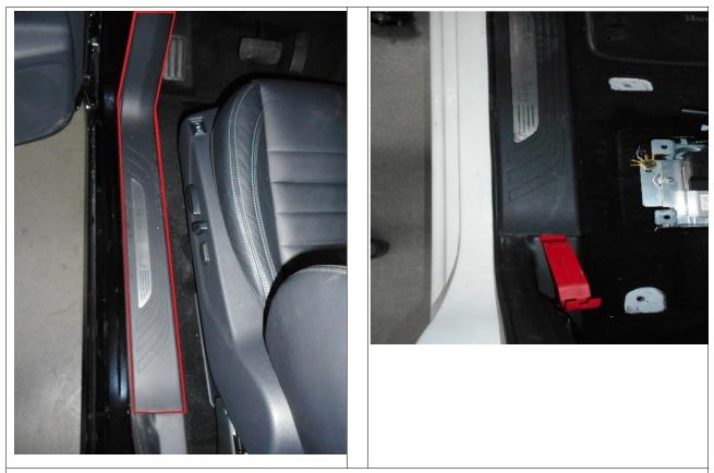
10. Remove the plastic sill protector by prising its rear part with an upholstery tool. Prise along the edge towards the front of the protector.
