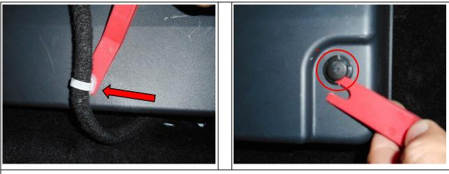
8. Prise the wires with an upholstery tool to remove them.9. Remove plastic pins mounting the cover, using an upholstery tool.
