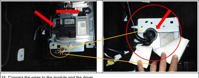
15. Connect the wires to the module and the driver.16. Lift the mat. Put the loudspeaker wire through the slot.
