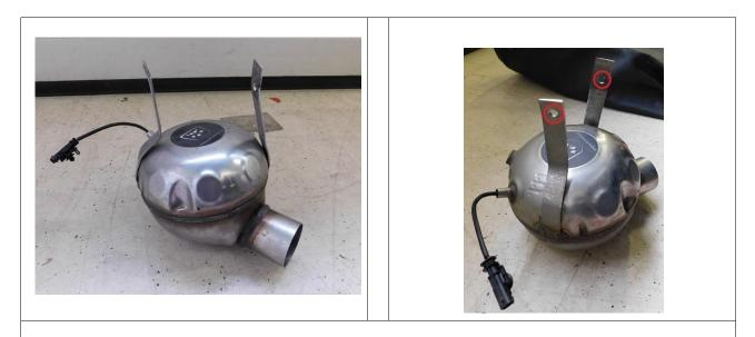
32. Fit and weld metal boards to the loudspeaker. Drill holes in each board to mount the loudspeaker in the car.
