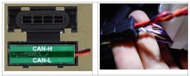
21. Fit the CAN reader to the wires:
