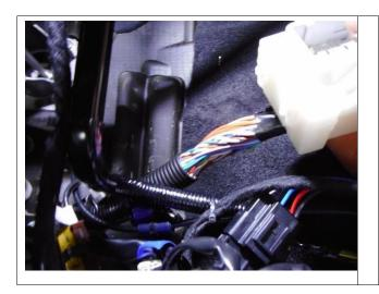
20. Remove the wire cover next to the removed plug. Find a blue and a pink CAN signal wire.
