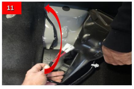
Guide the left and right main wiring through the console and behind the carpet. Route out under carpet to join factory seat wires. Tape together for support.
