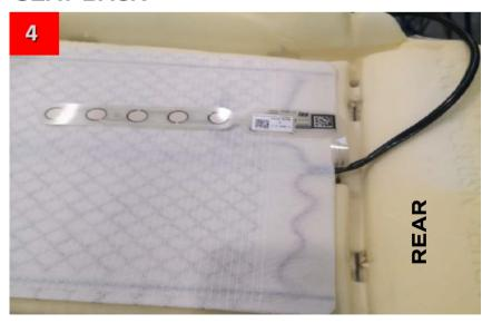
Align the 2nd heater pad on the base, as pictured, with the rear edge just in front of the occupancy sensor pad wire. (passenger seat)
