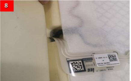
Guide the base heater pad wire through the hole along with sensor pad wire. Join with back wiring connector and cable tie in a secure position.
