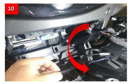
Insert the switch harness into the drilled holes, and guide wires to the cavity in front of gear lever.
