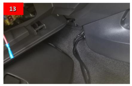
Power supply wires should be routed to the fuse panel, behind dash and carpet.
