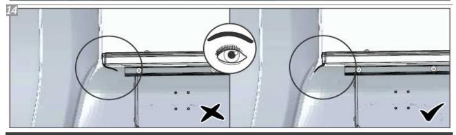
Ensure that the rubber flap is fitting over the front edge of the tray
