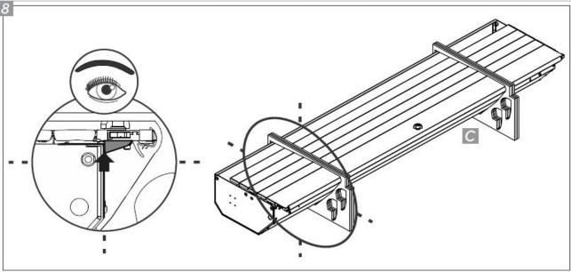
Ensure stop-wedge is on outside of the shutter cartridge (step 8)
