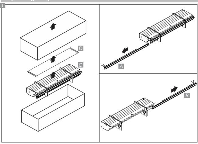
Be sure to keep the cardboard "ribs" on the shutter cartridge until step 11
