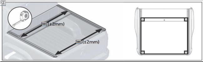
Measure the width between rails and ensure an even width. Adjust spacers as necessary.
