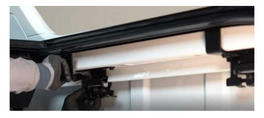
Adjust the position if the lid so that the holes match up to the factory tapped holes in the sailplane. Loosely insert all bolts before tightening. When tightening, start with the rear bolts as proper alignment is critical for correct operation of the shutterlid. (see next image for alignment notes).
