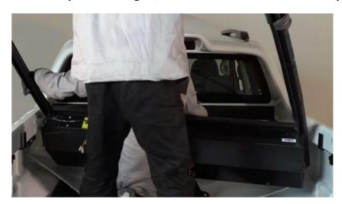
Place the rails on top of the installed rear brackets. Carefully lift the front of the lid unit and push toward front.
