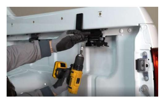
Fit the front bracket to the front of the tray and bolt down in place.
