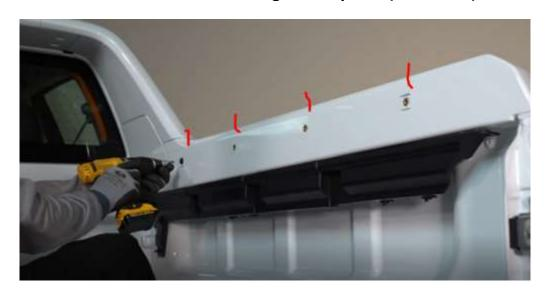
Remove trim panel by loosening bolts and removing clips that hold it in place
