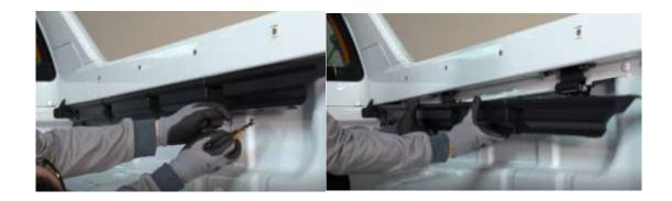
Remove the two front bolts of the rear clamp (LHS + RHS) as per picture.
