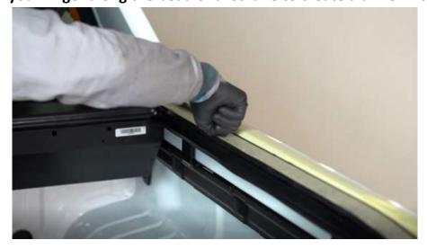
After allowing a surface set period of about 5 minutes, gently but evenly pull away the masking tape. Any excessive blotches must be cleaned up carefully before the urethane cures.
