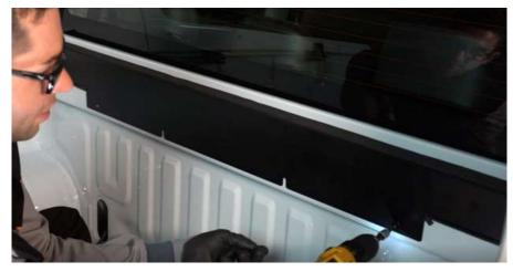
Apply urethane sealant all around the sides and bottom edge of the installed front bracket, ensuring to seal the entire seam. Also apply urethane to seal all gaps present between the sailplane and tray (see red line on image below)
