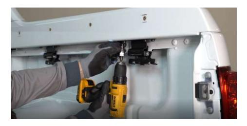
Bolt the bracket marked with a "T" (Tailgate side) using the bolts removed in the previous step.
