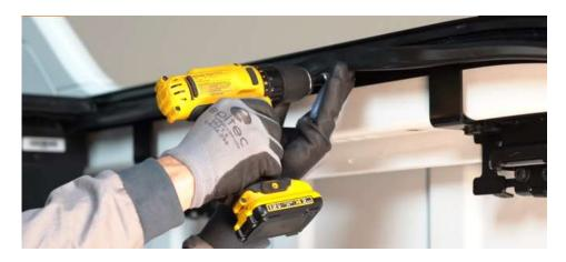
Close the tailgate and lift the shutterlid rail so that a gap of 2mm is present between the tailgate and the shutterlid rail bottom corner.
