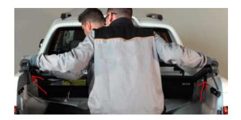
Lift the rubber on the front of the lid cover over the edge of the front tray bracket. Refer to step 14 of the standard instructions for correct orientation of this rubber. Incorrect fitment will result in excessive water leaks.
