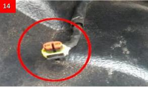
Connect the controller side connector to a power supply. Press both buttons on the controller for about 5 seconds until the light starts blinking.
