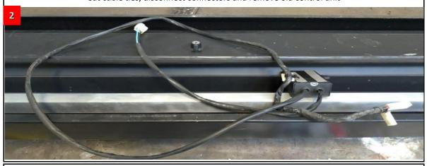
Locate the connector on the motor and cut the wires Thread the wires through the grommets, strip 4mm as close as possible to the connector off wire tips and crimp the pins to the wires.
