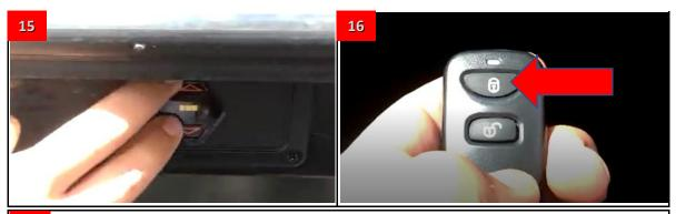
Disconnect test power source and repack cartridge and programmed remotes into box. Mark the box clearly with "NEW CONTROLLER INSTALLED & REMOTES PROGRAMMED"
