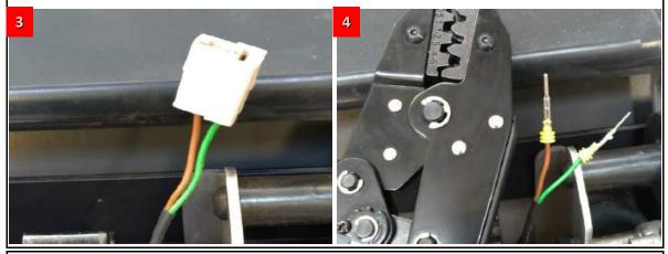
Note the numbers on the connectors and insert the pins accordingly (1-brown wire, 2-green wire)
