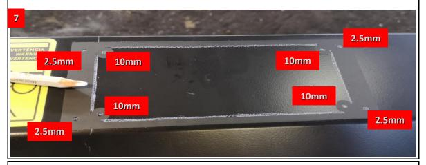
Use a +/-20mm holesaw to cut a hole large enough for the air-hacksaw blade to fit through. Cut out the inner block as per template.
